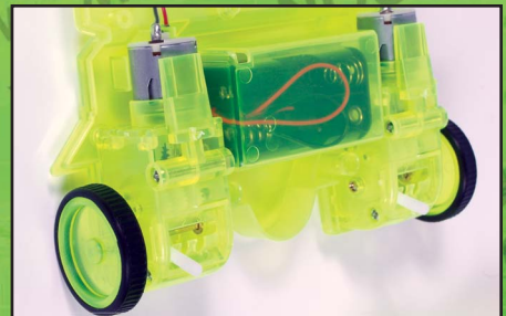
FIGURE 21. Mount the two motor gearboxes to the base plate. Make sure that the left and right gearboxes are installed on their correct locations. In this photograph, the left gearbox is at the top of the picture.
